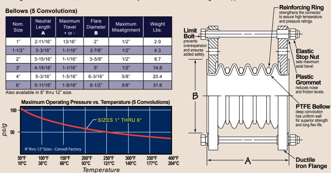
BlueLine™ flanges are ductile iron, drilled and tapped per ANSI B16.5 for Class 150 piping systems. Limitbolts are zinc-plated steel mounted through plastic grommets.
